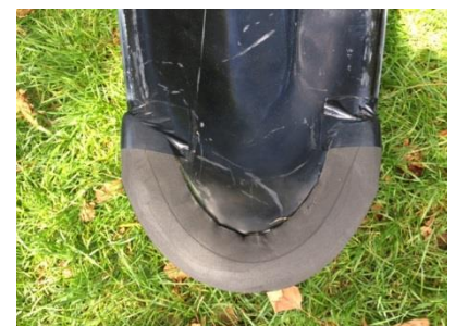
Pass- edge tape is ok as long as no gaps underneath
